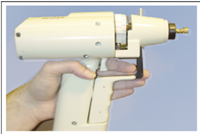
Figure 1. A gene gun. The Helios (Bio-Rad) gene gun is a small portable instrument that enables efficient transportation of dyes into cells – a technique that is becoming known as diolistics.
